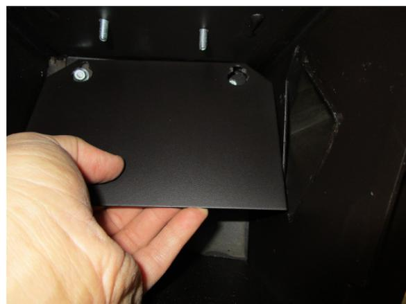
Fig. 97 - Flue gas deviator removal
