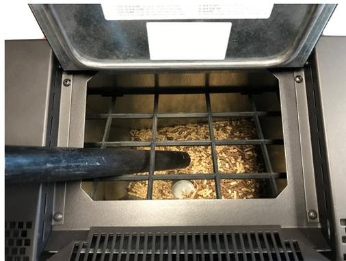
Fig. 91 - Hopper and auger cleaning
