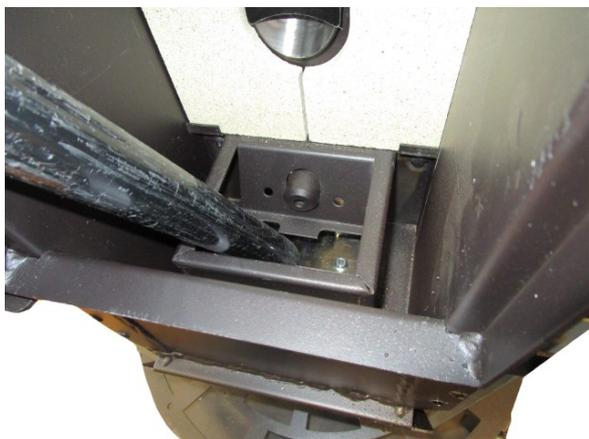
Fig. 89 - Burning pot box cleaning
