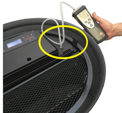
Fig. 68 - Digital pressure switch connection
