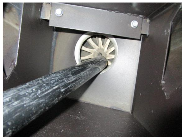
Fig. 99 - Vacuum out the ash
