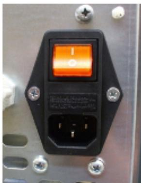
Fig. 66 - Electric socket with master switch
