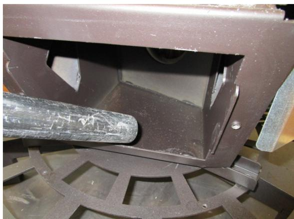
Fig. 98 - Vacuum out the ash
