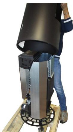
**Fig. 33 - Pull the drum off**
