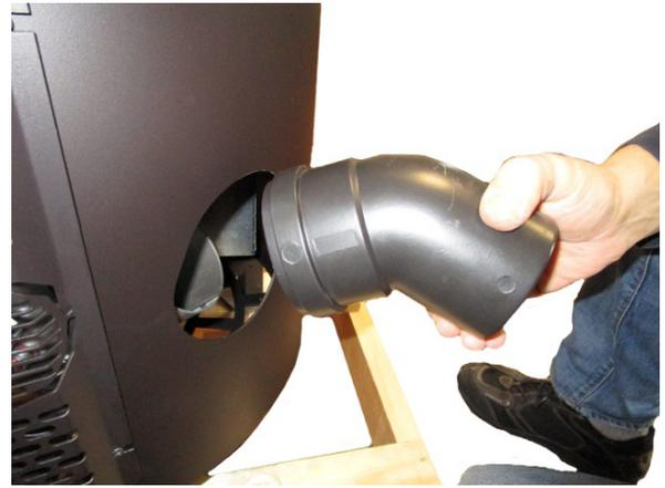
**Fig. 24 - Elbow removal**
