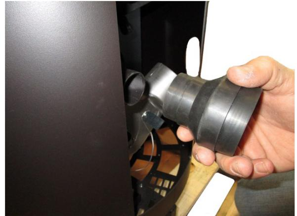
**Fig. 26 - Adapter removal**
