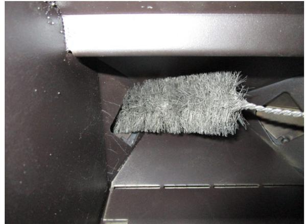
Fig. 103 - Cleaning with pipe cleaner 4
