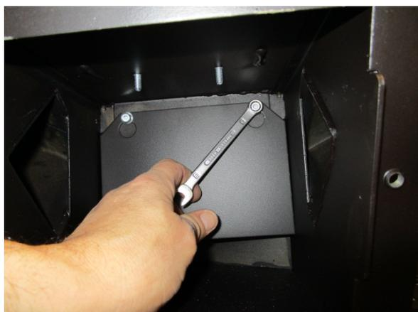
Fig. 96 - Screw removal
