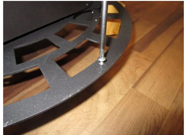
**Fig. 50 - Screw removal**
